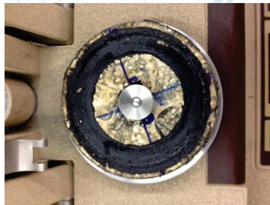
Asphalt Coated Galvanized Steel, 100 cycles
