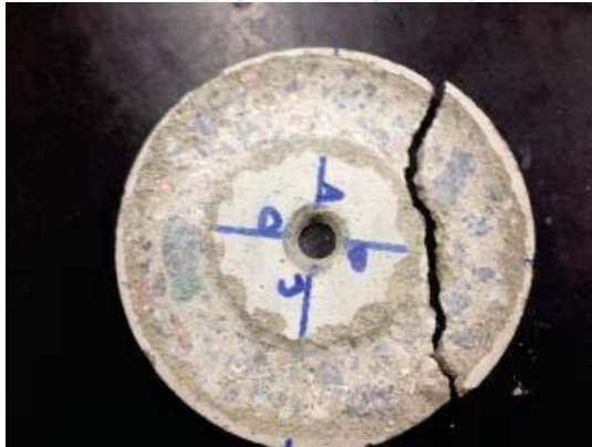
2400 psi Concrete, 4700 cycles
