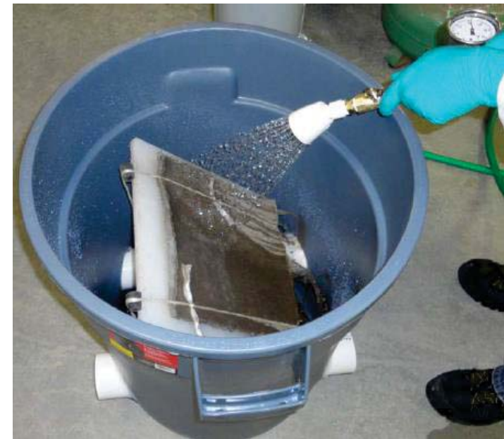
Hydration of initial samples with 1.25 gallons of water
