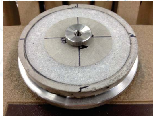
9300 psi Concrete, 5000 cycles
