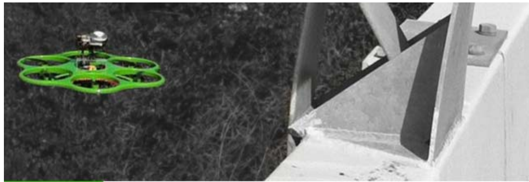
Hex copter Bridge Inspection Platform
